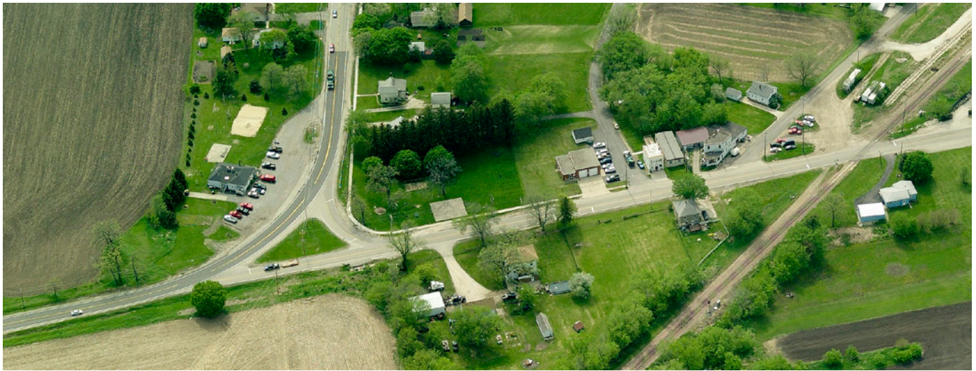
This photo shows the existing alignment of the U.S. Route 20 and Reinking intersection which is problematic due to the high speed of traffic approaching the curve and limited sight lines.
